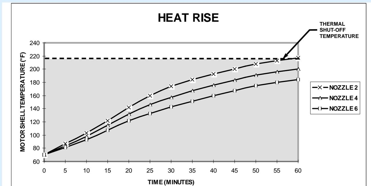
The motor driving this pump has a built in thermal protector that will open, shutting off the pump, when the surface temperature of the motor heats to approximately 215°F. Motors of this size and construction require 15 to 30 minutes of cooling time before the thermal protector closes and re-energizes the pump. Lower current levels heat more slowly, allowing longer run times, but the cool down time still averages about 30 minutes, at 70°F ambient temperature.
